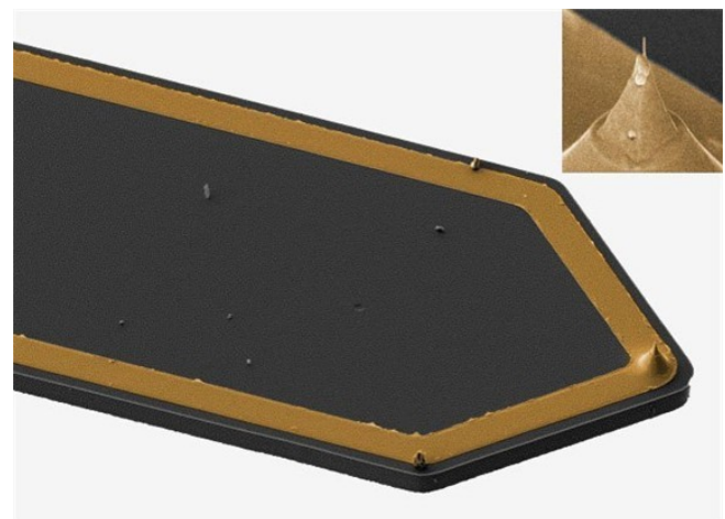
Conductive, self-sensing cantilever with a high aspect ratio conductive platinum tip featuring a tip radius < 20 nm
