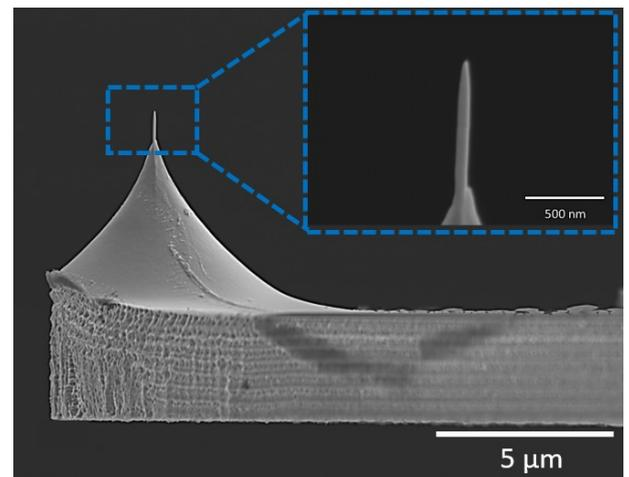
Magnetic „super-tip” fabricated by 3D nanoprinting for high resolution MFM imaging.
