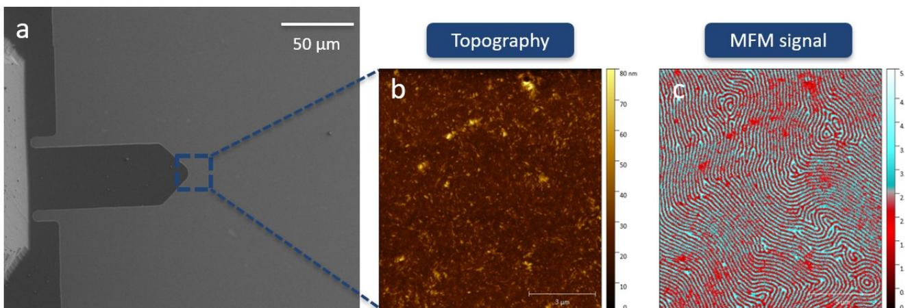
Topography and MFM measurements on a multilayer sample provided by L. Fallarino, G. Hlawacek, O. Hellwig (HZDR, Germany). (a) SEM guidance allows to find the region of interest. (b) AFM topography image of a smaller area and (c) the corresponding MFM signal measured with magnetic „super-tip”
