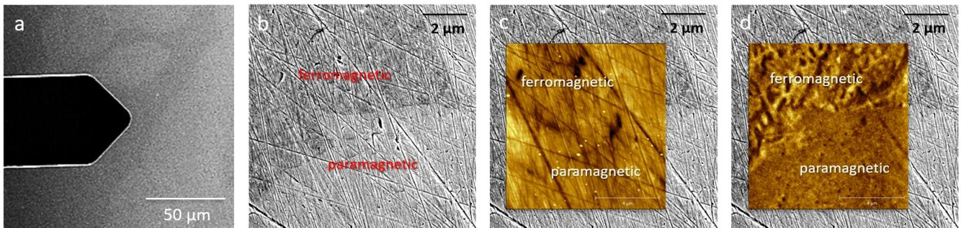
AFSEM® measurements of duplex steel sample provided by M. Knyazeva, J. Rozo Vasquez, F. Walther (TU Dortmund University). (a) SEM guidance allows the positioning of the cantilever on the region of interest. (b) SEM image with increased contrast shows ferromagnetic and paramagnetic phases. (c) Topography and (d) MFM signal.
